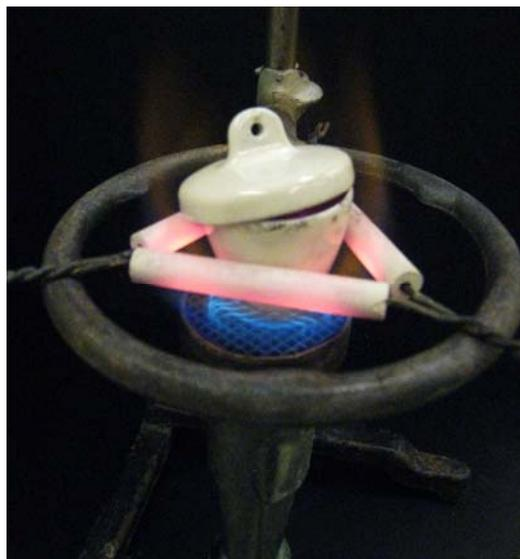
**Left:** Ashing the paper using a laboratory burner
