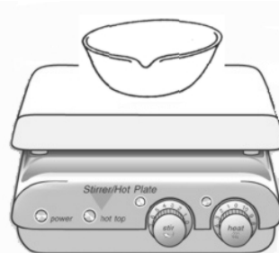
Figure 1. Heating an evaporating dish on a hot plate (left) and on a ring support (right).
