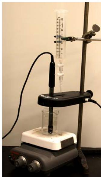
Figure 1. Drop counter setup
