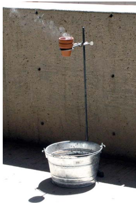
Figure 1. Apparatus for the thermite reaction.
