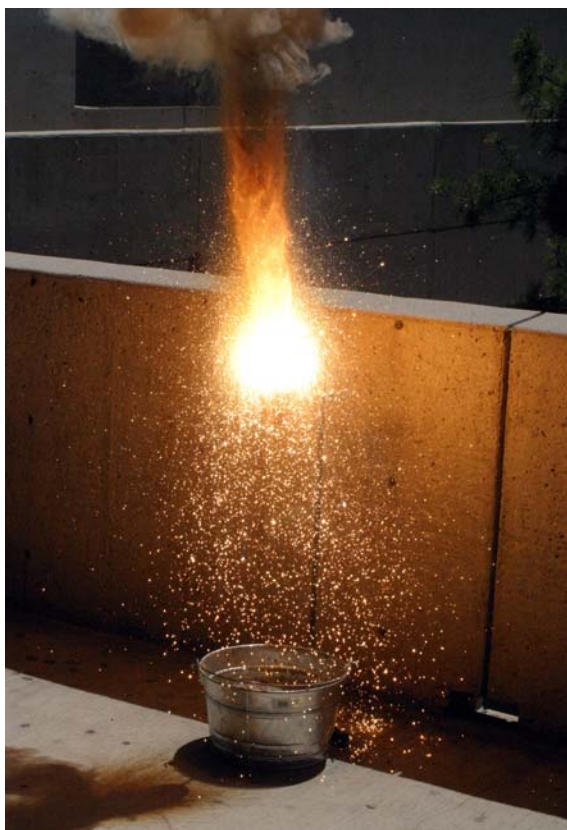
Figure 3. The thermite reaction.
