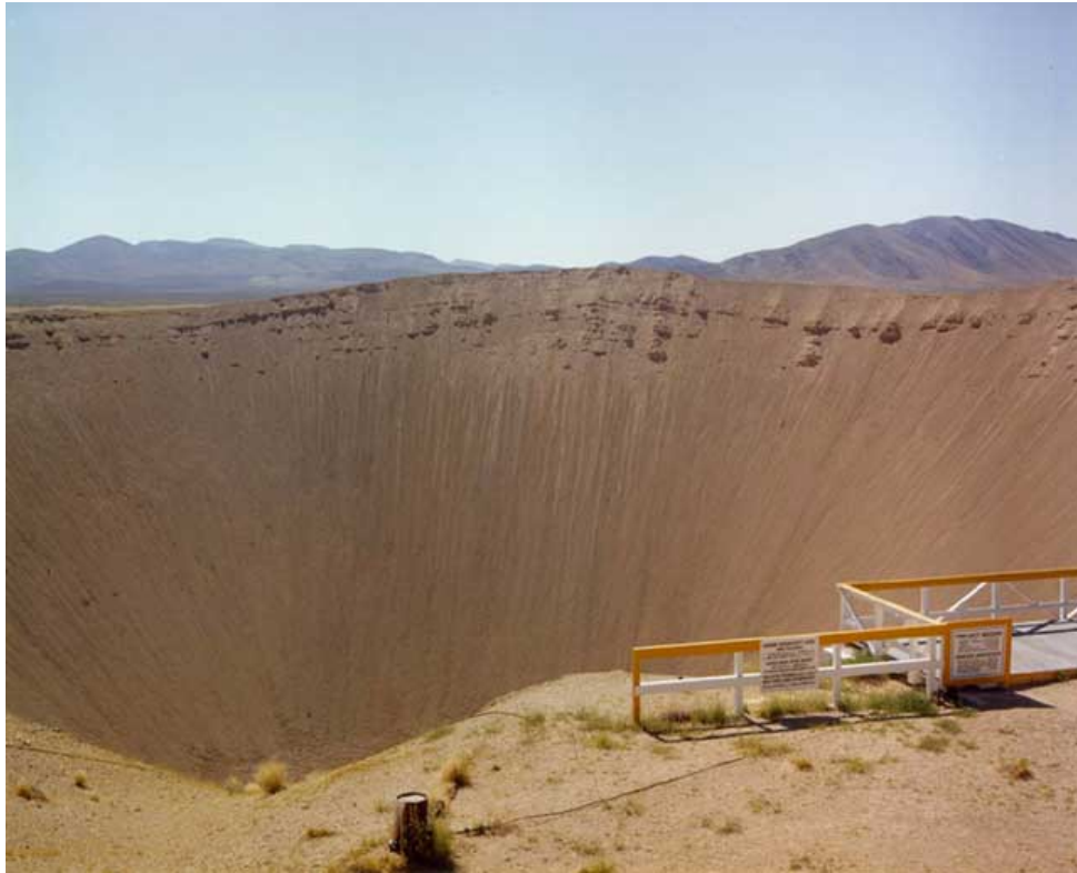
The 104-kiloton Sedan test in July 1962 left a crater 1,280 feet wide and 320 feet deep. (U.S. DEPARTMENT OF ENERGY)
