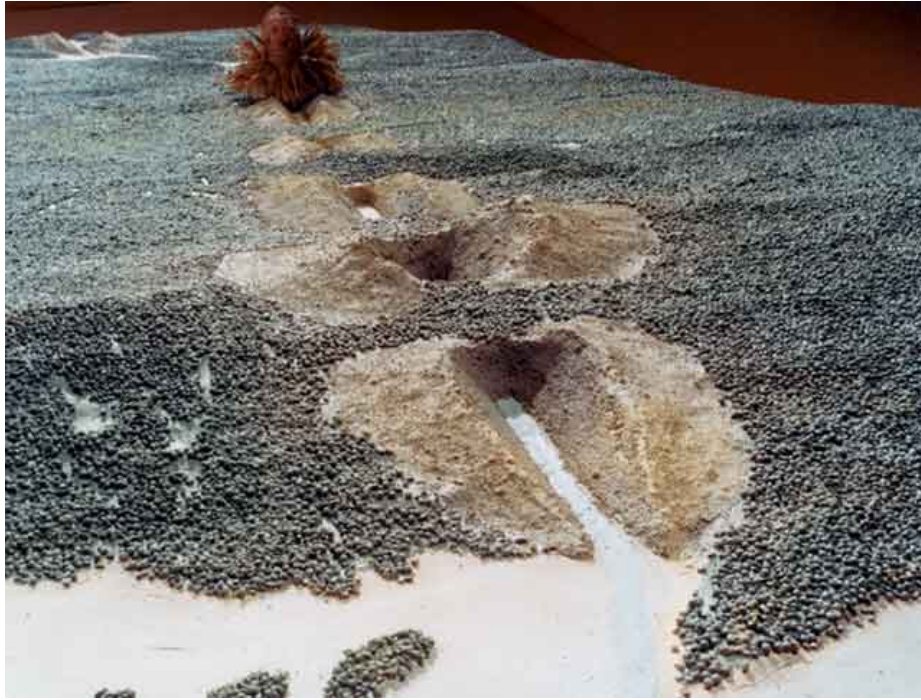
An engineers' model shows a series of detonations taking shape as a canal. (COURTESY OF LAWRENCE LIVERMORE NATIONAL LABORATORY)
