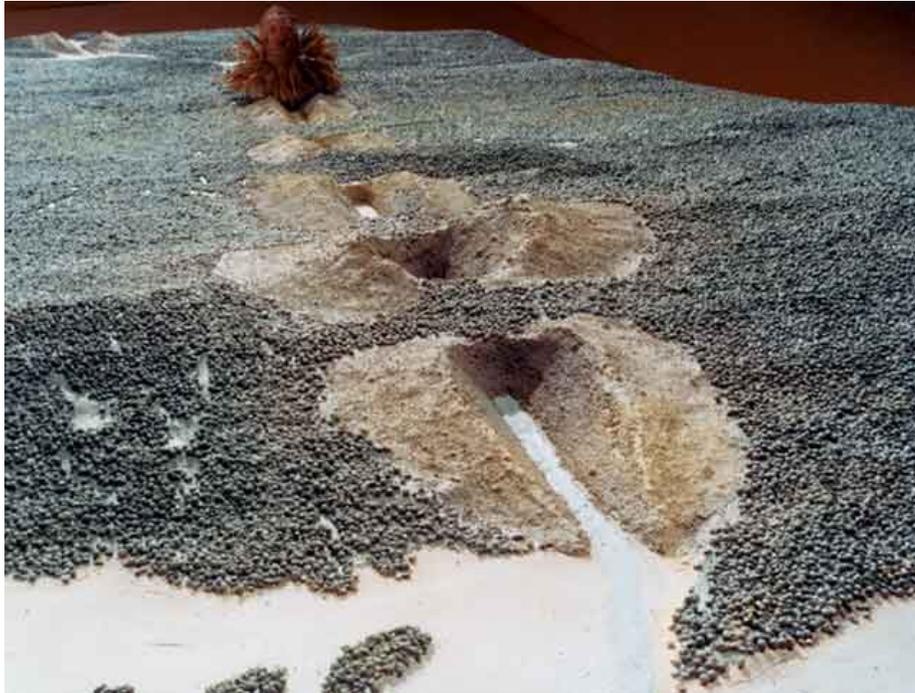
**An engineers' model shows a series of detonations taking shape as a canal.**
