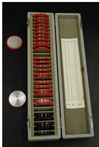
Shielding material set
