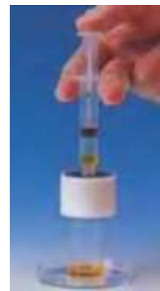
Figure 3. The ^{137}\text{Cs}/^{137}\text{Ba} Isogenerator
