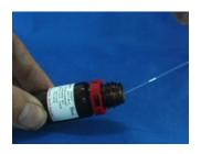
Use capillary action to transfer the 4'-pentyl-4-biphenyl-carbonitrile liquid crystal into a capillary tube.
