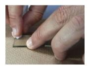
One edge of the glass must be free of PVA. Wipe about 2 to 3 mm of the PVA film off the edge by wiping with a damp tissue.
