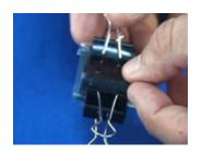
Add crossed polarizers, one on each side, slipping them under the binder clips.
