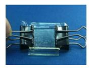
Clamp the glass squares together using binder clips.
