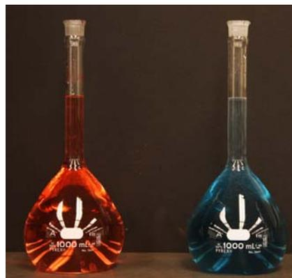
Place a large funnel in the top of the 2000-mL volumetric flask and pour the HCl and NaOH solutions into the larger flask. (The change in color will indicate mixing/reaction.) Note the volume of the solution. What is the final volume? (You can measure the final increase in volume using a graduated cylinder. Note: The volume will be slightly increased due to the warm solution. For an accurate measurement of the volume increase, allow the solution to cool to room temperature.)
