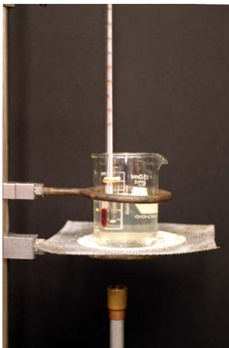
Figure 2. Micro boiling point apparatus with detail shown on the right. (The thermometer is supported by a thermometer clamp.)
