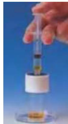
**Figure 3.** The  $^{137}\text{Cs}/^{137}\text{Ba}$  Isogenerator
