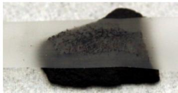
Place approximately half of the tape onto the graphite sample.
