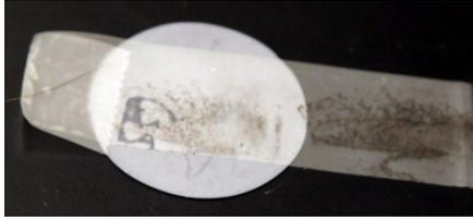
Place the tape with the last graphite layer onto a silicon disk. Take care as the silicon wafers are fragile and break easily.
