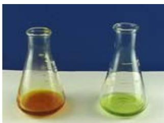
The iron solutions need to be completely dissolved, well sealed and free of any particles. Color is important! Fe(II) is air sensitive. 1M  $\text{FeCl}_3$  in 2 M HCl (shown at left) 2 M  $\text{FeCl}_2$  in 2 M HCl (shown at right)
