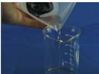
Use a strong magnet to attract the ferrofluid to the bottom of the weighing boat. Pour off and discard as much clear liquid as possible. Rinse again with water from a wash bottle and discard the rinse as before. Repeat the rinsing a third time.
