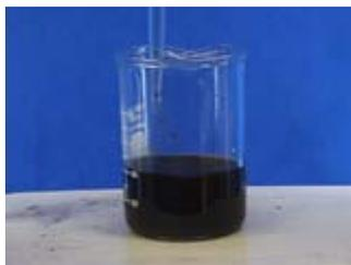
With continued stirring, use a dropper to add 50 mL of 1.0 M aqueous  $\text{NH}_3$  solution slowly over a period of 5 minutes. After an initial brown precipitate, a black precipitate will form (magnetite). (Slow addition of the ammonia solution can also be accomplished using a buret or separatory funnel.)
