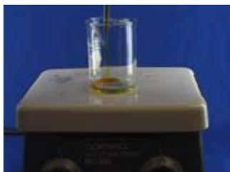
Add 4.0 mL of 1M  $\text{FeCl}_3$  and 1.0 mL of 2M  $\text{FeCl}_2$  solution to a 100 mL beaker. Add a magnetic stirring bar and begin stirring.
