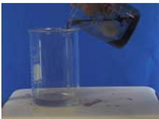
Let the magnetite settle, then decant (pour off) and discard the clear liquid without losing a substantial amount of solid. You can speed the settling process by putting a magnet under the container.
