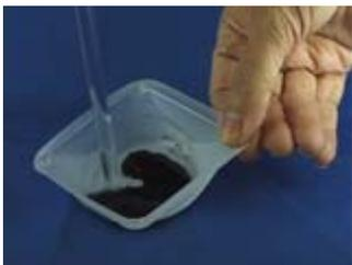
Add 1-2 mL of 25% tetramethylammonium hydroxide. Gently stir with a glass rod for at least a minute to suspend the solid in the liquid. Use a strong magnet to attract the ferrofluid to the bottom of the weighing boat. Pour off and discard the dark liquid. Move the strong magnet around and again pour off any liquid. If the ferrofluid does not spike, continue to move the strong magnet around, pouring off any liquid.
