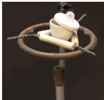
Figure 1. Heating a crucible
